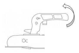
Place hitch lock in coupling (side notch towards handle)
