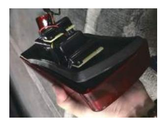
**Step 5.** Unplug the green/black wire of the load resistor on the LED tail light. Failure to do so will cause a dashboard error warning.
