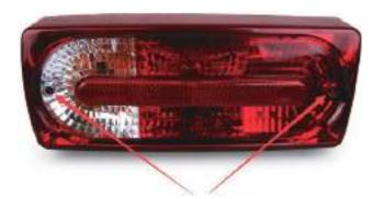
Remove the two screws, then take off the taillights lens
