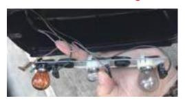
Brown wire is ground/negative pole-Gray/Red wire is taillight+ Black wire is brake light+ Green/Black wire is turn signal light+
