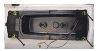
**Step 4.** Take off the black plastic gasket from the original taillights, then insert the black gasket into the new LED taillights.
