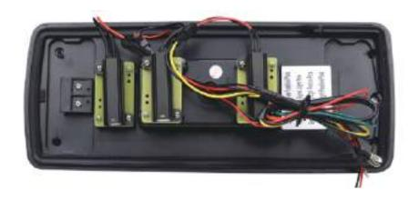
Step 6. Connect the wires before you secure the LED taillights assembly.
