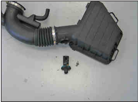
16. Install the provided gasket onto the mass air sensor adapter. NOTE: Vehicle's MAF sensor may vary among model years, use appropriate gasket and mass air sensor adapter.
