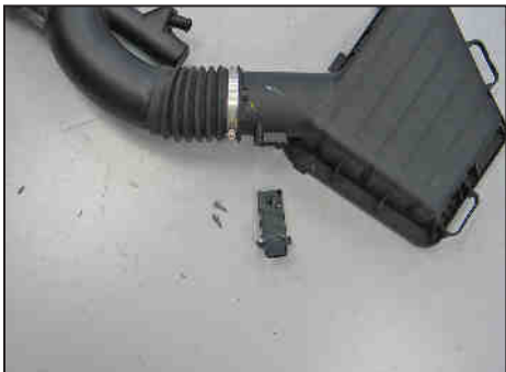
17. Remove the two screws that secure the mass air sensor into the factory intake tube. NOTE: Vehicle's MAF sensor may vary among model years, reference appropriate image above.
