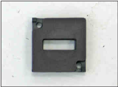
16. Install the provided gasket onto the mass air sensor adapter. NOTE: Vehicle's MAF sensor may vary among model years, use appropriate gasket and mass air sensor adapter.
