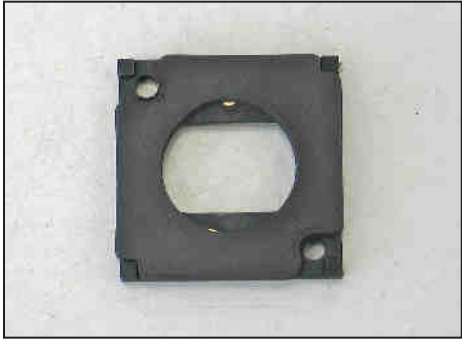
15. Install the heat shield assembly into the vehicle so the inserted nut goes into the air box mounting grommet hole and the tab goes onto the air box mounting stud. Secure the heat shield with the provided hardware.
