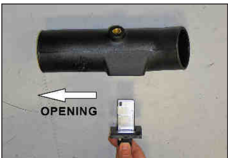
19. Install the mass air sensor assembly into the K&N® intake tube as shown and secure with the provided hardware. NOTE: The opening of the mass air sensor is to be pointed towards the inlet side of the tube as shown in photo. NOTE: Vehicle's MAF sensor may vary among model years, reference appropriate image above.
