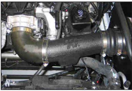
21. Install the provided silicone hose (08629) onto the K&N® intake tube as shown. Install the K&N® intake tube assembly onto the throttle body and hump hose attached to the filter adapter. Adjust the intake tube in the hoses for proper fit, once proper fit is achieved secure the tube with the provided hose clamps.
