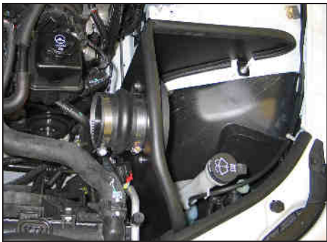
15. Install the heat shield assembly into the vehicle so the inserted nut goes into the air box mounting grommet hole and the tab goes onto the air box mounting stud. Secure the heat shield with the provided hardware.
