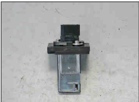
18. Install the mass air sensor into the mass air sensor adapter and secure with the provided hardware. NOTE: Vehicle's MAF sensor may vary among model years, reference appropriate image above.
