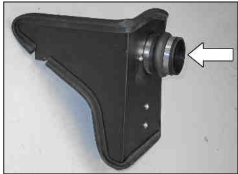
14. Install the provided silicone hose (5-576) onto the filter adapter as shown and secure with the provided hose clamp.
