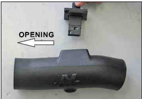
18. Install the mass air sensor into the mass air sensor adapter and secure with the provided hardware. NOTE: Vehicle's MAF sensor may vary among model years, reference appropriate image above.
