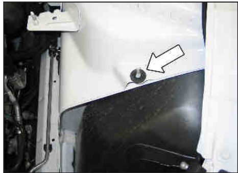
13. Install the provided rubber fender washer onto the outer air box mounting stud.
