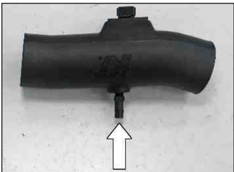
20. Install the provided vent fitting into the K&N® intake tube as shown. NOTE: Plastic NPT fittings are easy to cross thread. Install the vent fitting "hand" tight, then turn it two complete turns with a wrench.
