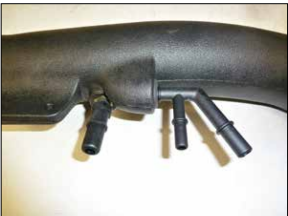
19. Install the remaining CCV fitting into the K&N intake tube as shown. Install the provided ejector fitting into the K&N intake tube using the provided grommet.
