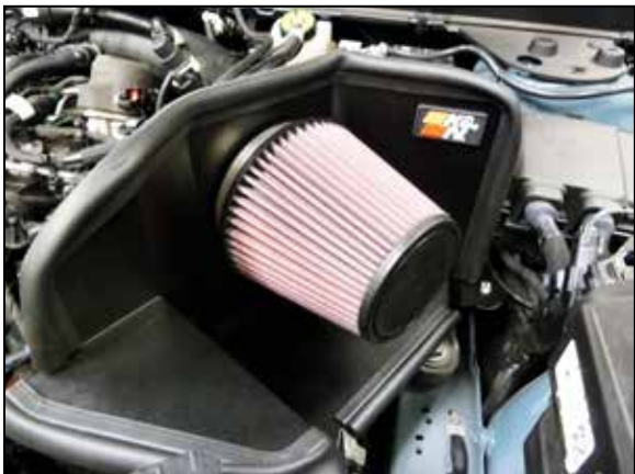
26. Install the K&N air filter and secure with the provided hose clamp.
