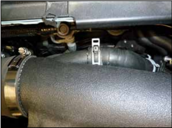
21. Connect the BOV hose too the K&N intake tube and secure with the factory spring clamp.
