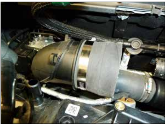
17. Install the provided step coupler onto the turbo inlet and secure with the provided hose clamp.
