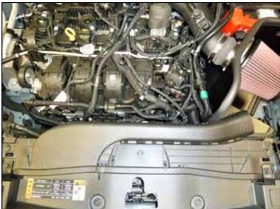
27. Reinstall the factory fresh air duct and secure with the factory pushpins.
