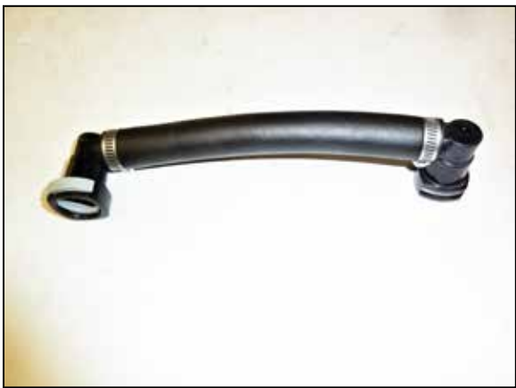
22. Assemble the provided CCV fittings and hose as shown.
