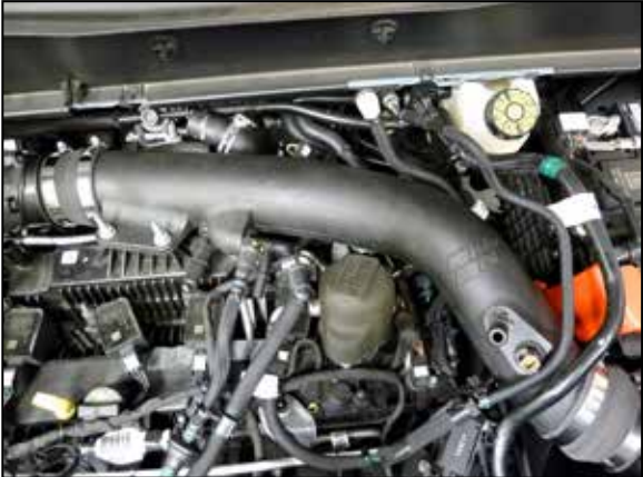
20. Install the K&N intake tube into the couplers at the filter adapter and turbo inlet, adjust the tube for best fit and secure with the provided hose clamp and factory hardware.
