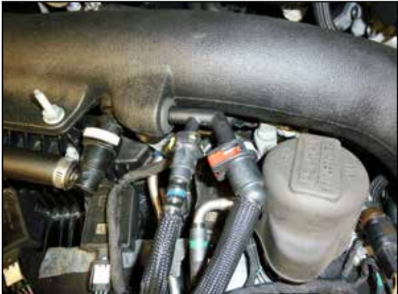
24. Connect the ejector line fittings to the ejector and secure the factory retaining locks.
