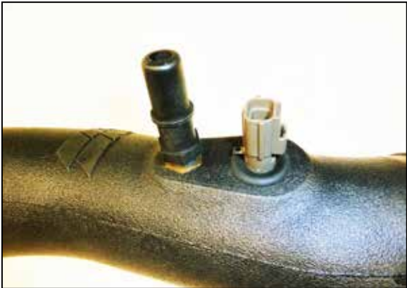
18. Remove the IAT sensor from the factory air filter housing, remove the O-ring from the sensor and then install the sensor into the K&N intake tube using the provided grommet. Install the provided CCV fitting into the K&N intake tube. NOTE: The IAT sensor is fragile, use caution while handling the sensor. NOTE: On models may not be equipped with this vent line, skip to the next step.
