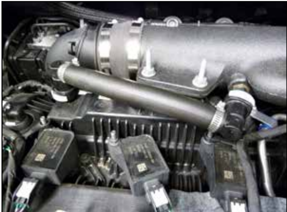
23. Install the CCV assembly onto the valve cover port and the fitting installed into the K&N intake tube.
