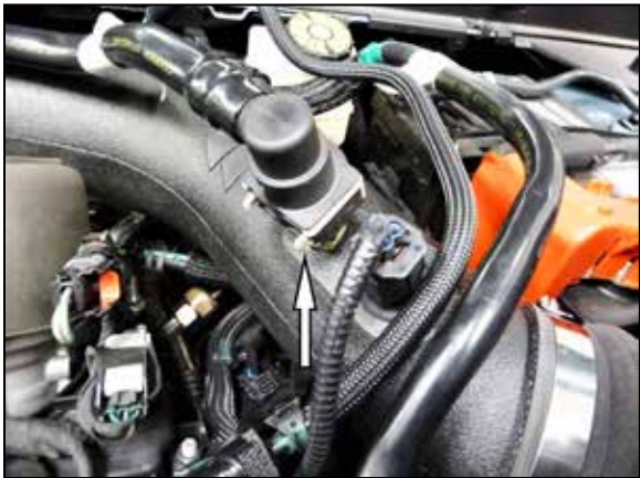
25. Reinstall the factory vent, secure the safety lock and reconnect the electrical connection. NOTE: On models may not be equipped with this vent line, skip to the next step.
