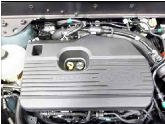
28. Reinstall the engine cover and secure with the factory hardware.
