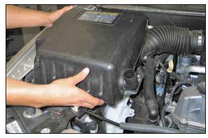
5. Remove the upper air box cover as shown.
