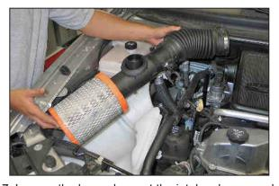
7. Loosen the hose clamp at the intake plenum and then remove the complete intake system.
