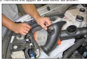
6. Remove the fresh air supply duct.
