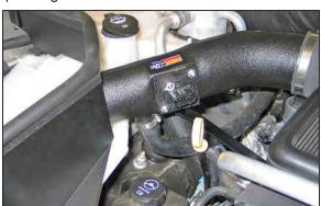
19. Cut the air injection hose at the location marked in step #18. Then install the hose onto the K&N® intake tube and secure with the provided hose clamp.
