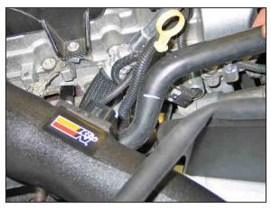
18. Mark the air injection hose at the base of the top 90deg bend as shown.
