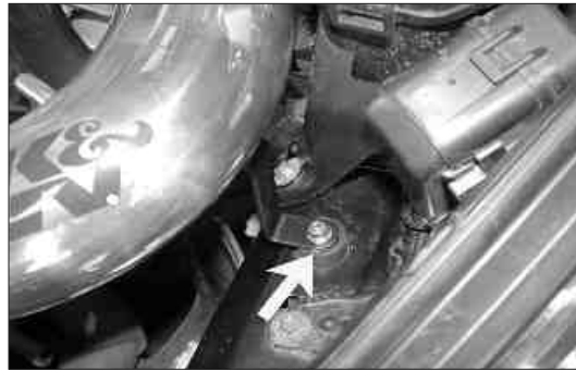
36. Line up the "Z" bracket with the rubber mounted stud and secure it with the provided hardware as shown.
