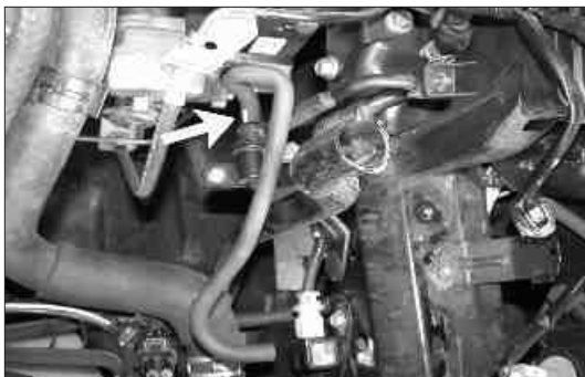
33. Reconnect the vent hose removed in step 23 to the EVAP OBD canister closed valve as shown.
