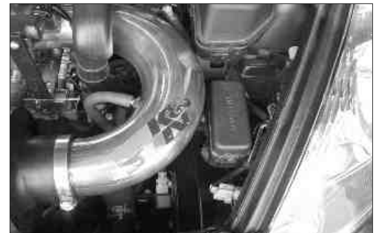
45. Slide the relay and fuse box back onto the stock bracket as shown.
