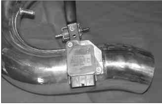
28. Install the mass air sensor into the intake tube and secure using the provided hardware as shown.
