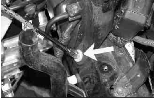
29. Loosen and remove the stock nut on the relay and fuse box support bracket as shown.
