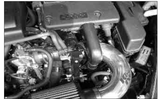
44. Install the computer fresh air tube as shown.
