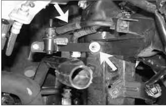
31. Install the EVAP OBD canister closed valve assembly into the vehicle and connect the hose to the hard line, then, secure the bracket to the relay and fuse box support bracket using the nut removed in step 29.
