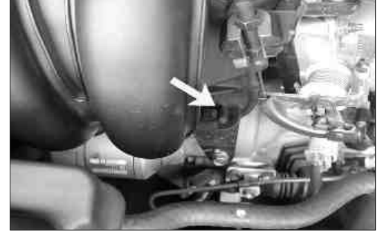
41. Cap the vent on the intake manifold using the provided rubber plug as shown.
