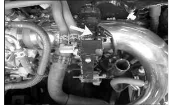
40. Reconnect the PWM vacuum switching valve electrical connection as shown.
