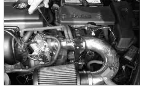
43. Adjust the tube for best fit and clearance and tighten all hardware and hose clamps as shown.
