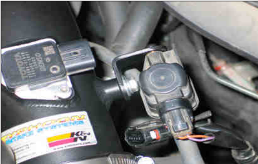
34. Secure the "L" bracket and pulse width modulated (PWM) switching valve assembly to the intake tube using the provided hardware.
