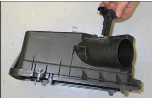
28. Remove the two screws that secure the mass air sensor to the air box. Remove the mass air sensor.
