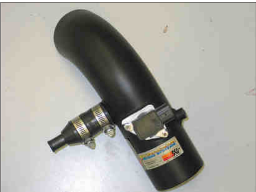
29. Install the stock mass air sensor into the intake tube and secure with the provided hardware.
