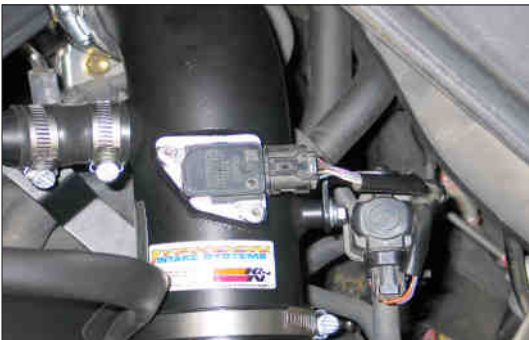
35. Re-connect the mass air sensor electrical connection.
