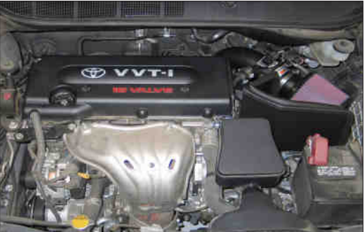
36. Reconnect the vehicle's negative battery cable. Double check to make sure everything is tight and properly positioned before starting the vehicle. 37. It will be necessary for all K&N® high flow intake systems to be checked periodically for realignment, clearance and tightening of all connections. Failure to follow the above instructions or proper maintenance may void warranty.
