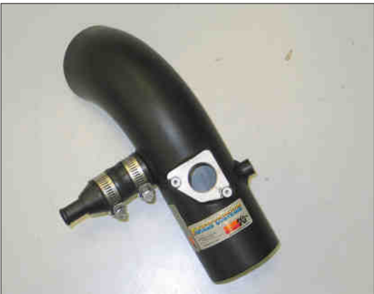
27. Install the stock crank case vent chamber into the silicone hose installed onto the intake tube secure with the provided hose clamp.
