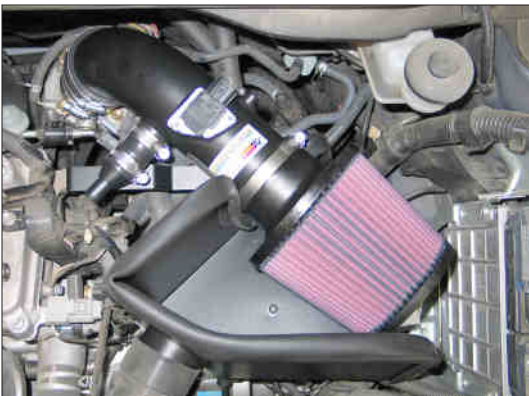
31. Install the intake tube assembly into the silicone hose installed onto the throttle body. Align with the intake tube mounting bracket installed in step # 16; then, secure the intake tube assembly using the provided hose clamp and hardware.
